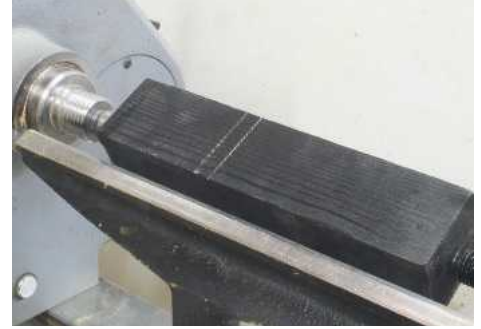
▲ Pic.6 I have sprayed a piece of pine black to make it easier to see the cuts I've made. I have marked the area that will be cut in from the square to the round
